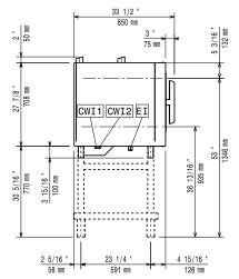
Cold Water inlet 1 (cleaning) CWII = Cold Water Inlet 2 (steam generator) CWI2
